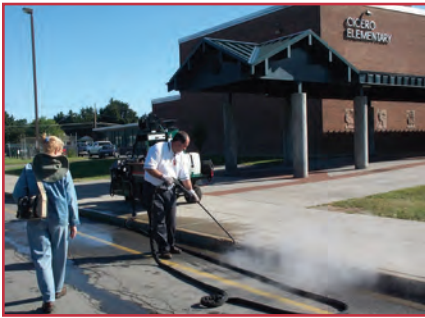
The latest in IPM: Hot water machines kill weeds without herbicide.
